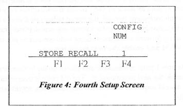
The final setup screen is used to store and recall user configurations is shown in figure 4. To enter this screen from setup screen 3, press the SETUP and up arrow keys simultaneously.
