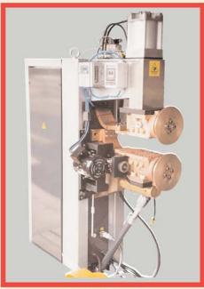
SEAM WELDER MODEL WT-SW-100 Inverter type control for precise control of acceleration and speed during welding. Wheels start rotating after they contacted the part and pressure is built up.
